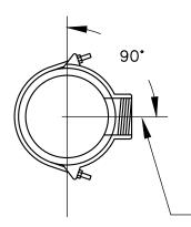
2" TAPS FOR 1 1/2" AND 2" DIA. SERVICES SHALL BE MADE UTILIZING A TWO STRAP TAPPING SADDLE, HAVING IP THREADS. TAPPING SHALL BE DONE WITH A MUELLER MODEL D-5 TAPPING MACHINE ALL IN ACCORDANCE WITH THE INSTRUCTIONS INCLUDED WITH SAID TAPPING MACHINE.
