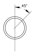
TAPS FOR 1" DIA. SERVICES SHALL BE MADE UTILIZING A MUELLER MODEL B-101 TAPPING MACHINE. THREADS SHALL BE CC. TAPS SHALL BE IN ACCORDANCE WITH THE INSTRUCTIONS INCLUDED WITH SAID TAPPING MACHINE.
