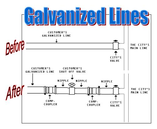
**Regulations:** *Valve* must be installed at least ONE (1) foot from the City's *Valve*, unless for some reason there is some type of obstacle that would prevent it; cement, shed, etc. Keep in mind you are still responsible for the line in between the City's *Valve* and your *New Valve*; if a break occurs between the Valves, the customer will still be charged \$25 for the Service Call ... so try not to get too far away.
