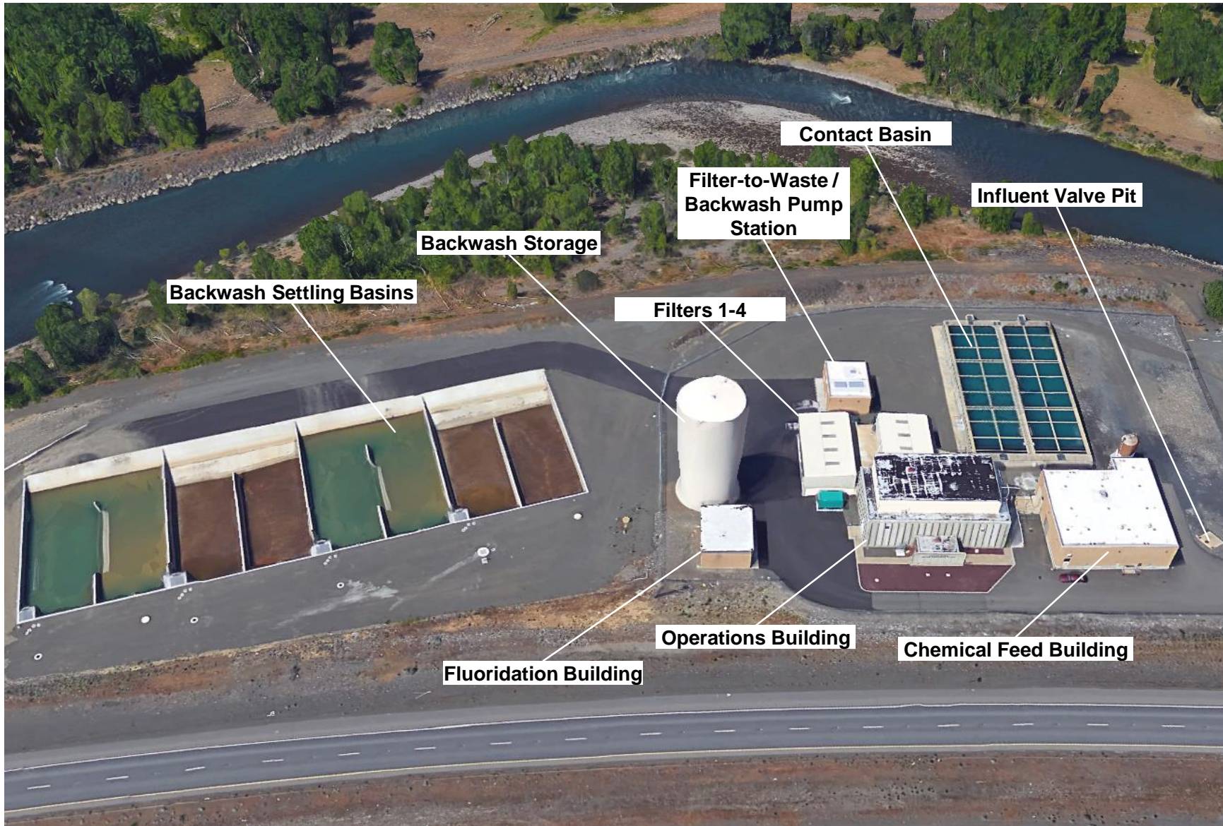
Figure 3-4 Naches Water Treatment Plant Site Plan
