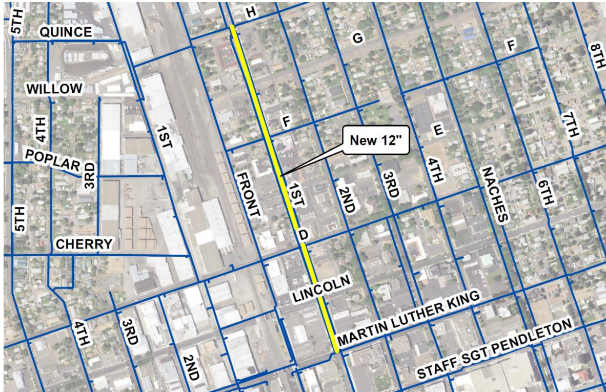
Figure 3-43. North 1 st Street Waterline Improvements - Phase 3
